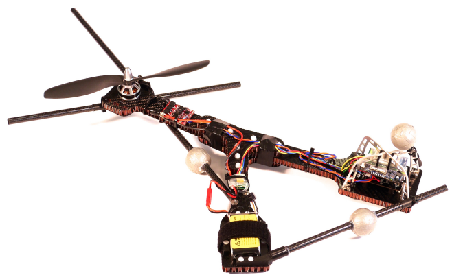
Fig. 1. The monospinner: a controllable flying vehicle with a single moving part. The vehicle is approximately 40 cm in size, the frame consists of five carbon-fiber plates, and the electronics are mounted in an aluminium cage inspired by the AscTec Hummingbird [12]. The carbon fiber rods help to protect the propeller during landing. A more detailed list of components is given in Table I.
