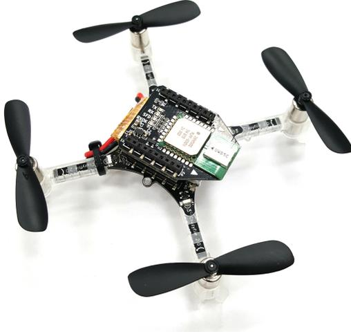
Fig. 3. The quadcopter used in our experiments as the mobile agent. <sup>†</sup> UWB ranging sensor (sees in this picture) works at the rate of approximately 60 Hz.
