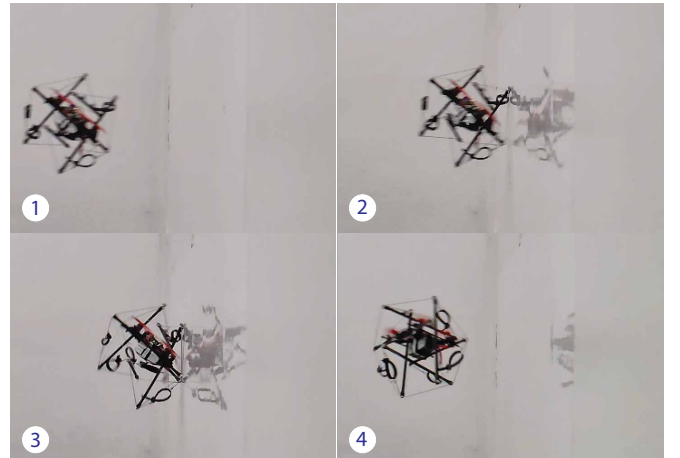
Fig. 6: Video sequences of the collision process: 1) Vehicle accelerates towards the wall. 2) Collision starts. 3) Vehicle comes to a full stop. 4) Vehicle bounces back from the wall. The speed of the vehicle right before the collision is 6.5m/s.
