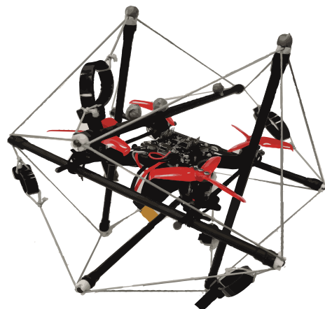
Fig. 1: The icosahedron structured aerial vehicle. The length of each rod in the icosahedron tensegrity shell is 20cm.
