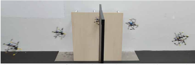
Fig. 7: Image sequence of the tracking experiment. The multicopter tracks a trajectory from left to right while avoiding the black obstacle in the middle of the space. For the collision-inclusive trajectory, the multicopter takes advantage of a collision with the yellow obstacle in the back. The distance between the shown left-most state and right-most state is about 2m.
