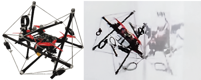
Fig. 1: The collision-resilient tensegrity multicopter (left) can still operate after colliding with a concrete wall with speed up to 6.5m/s (right). We use it as a test platform for the collision-inclusive planner.
