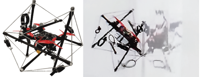
Fig. 1: The collision-resilient tensegrity multicopter (left) can still operate after colliding with a concrete wall with speed up to 6.5m/s (right). We use it as a test platform for the collision-inclusive planner.
