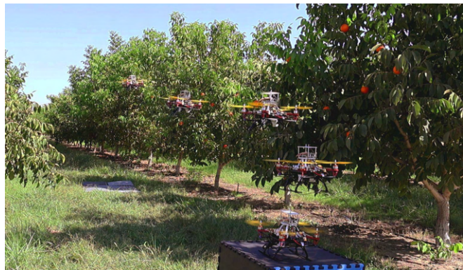
Fig. 1. Experimental vehicle flying autonomously at canopy level while collecting visual data using a RGB camera. This figure is a compound image showing multiple states of the vehicle during flight.
