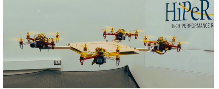
Fig. 1: Four quadcopters cooperatively carrying a single panel payload.
