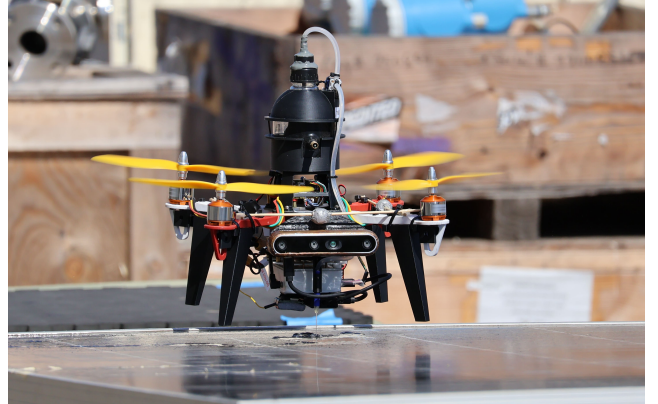
Fig. 1. The quadcopter flying over a 1.1 \times 2.3 m photovoltaic panel, showing the reservoir mounted on top and the liquid being dispersed through a jet nozzle mounted at the bottom.
