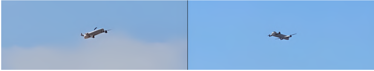
Figure 4.17: Outdoor flight footage of the drone operating in two different control modes. Left: conventional quadcopter mode, where the rotors are fixed upright to the vehicle body, and the vehicle pitches forward during forward flight. Right: PairTilt mode, where the vehicle body is commanded to remain level, and the rotors tilt forward to generate forward thrust. Both photos show the vehicle flying at 15 m/s. Despite the same speed, the conventional quadcopter mode exhibits a much larger pitch angle, resulting in higher air resistance and power consumption.
