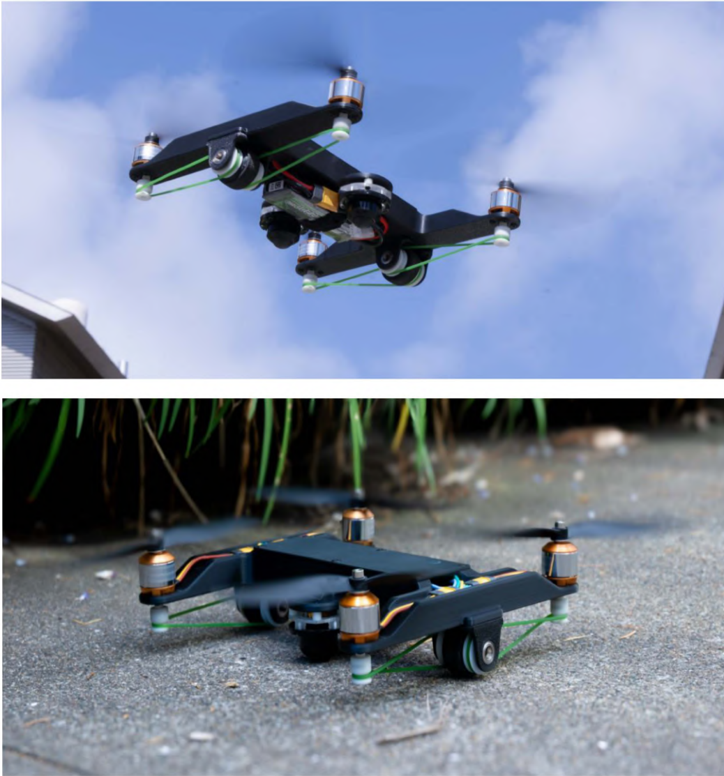
Figure 5.1: Top: Duawlfm is in aerial mode. Bottom: Duawlfm is running on the sidewalk in ground mode.
