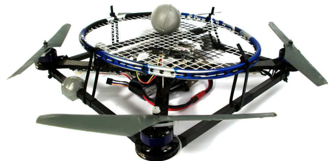
Fig. 1. A quadrocopter with attached badminton racket head. Three retro-reflective markers are attached to the vehicle, with which the vehicle pose can be determined (here, two are partially obscured by the racket). The ball, shown lying on the racket, is also wrapped in the retro-reflective tape to be visible to the motion capture system.
