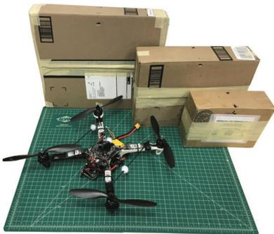
Fig. 6. Hardware used for the experimental results. The quadcopter weights approximately 0.7 kg; the radius of each propeller is 0.1 m. The largest surface of each box is approximately 0.114 m<sup>2</sup>, 0.082 m<sup>2</sup> and 0.054 m<sup>2</sup>.
