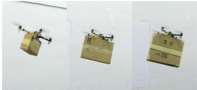
Fig. 1. Quadcopter carrying different payloads with similar mass but different size. The proposed control scheme finds the speed that maximizes the range of the vehicle along a given path. It adapts to unknown disturbances, such as the aerodynamic interference from a payload.
