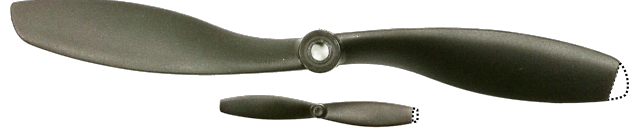
Fig. 3. The damaged propellers used in the experiments, with the removed propeller sections indicated by dashed outlines, on the right-hand side. The damage to the small propeller is approximately 5mg, and that to the large propeller is approximately 40mg.
