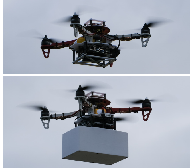
Figure 1. A quadcopter carrying payloads with differing mass and aerodynamics properties, as used in our experiments.
