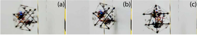
Figure 9. Sequence of images showing the process of a collision against a concrete wall: (a) Vehicle accelerates towards the wall. (b) Vehicle comes to a full stop. (c) Vehicle bounces back from the wall. The collision speed is 7.8m/s.
