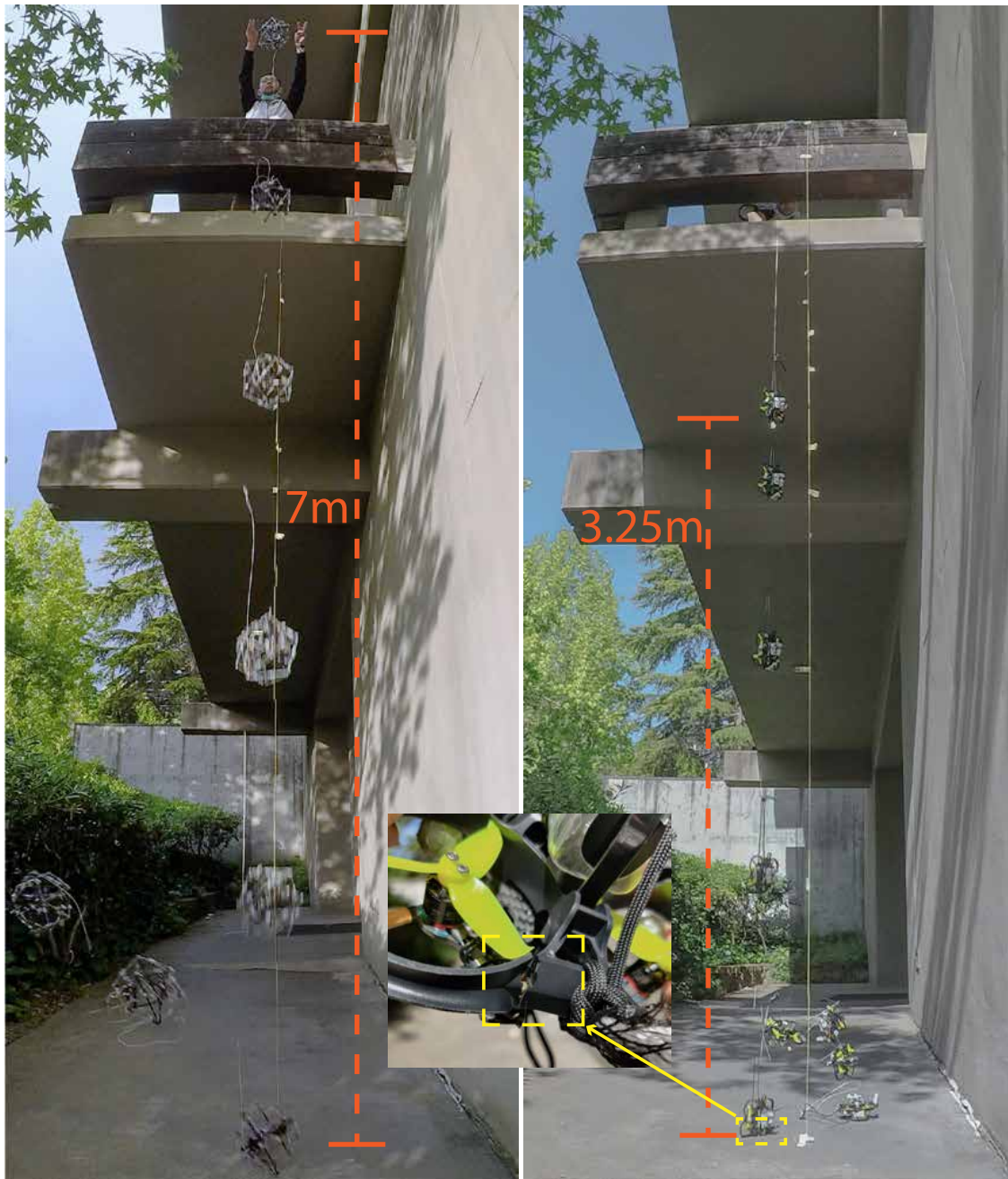
Figure 3.9: Composite image of the drop experiments validating the collision resilience of the experimental vehicle. Left: the experimental vehicle survives a 7m drop with a landing speed of 11.7m/s. Right: for comparison, the quadcopter hosting same electronics and propellers, built with commercial propeller guard, fractures after a 3.25m drop with a landing speed of 8m/s. The fracture is highlighted with the yellow box.
