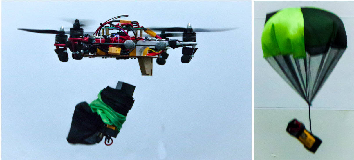
Figure 3.1: (Left:) Quadcopter dropping its first stage after use. A parachute is attached to the ejected stage to avoid damage to the battery or the surroundings. (Right:) Ejected stage with the deployed parachute.
