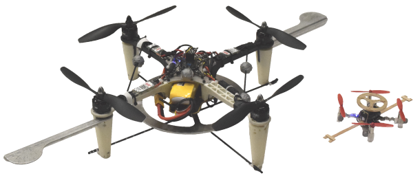
Fig. 6 Test vehicles with attached arm extensions. A falling mass collides with the arm extension in order to provide an torque impulse disturbance to the vehicle.
