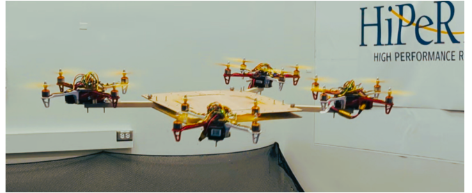
Fig. 1: Picture of four drones cooperatively carrying a single panel payload.
