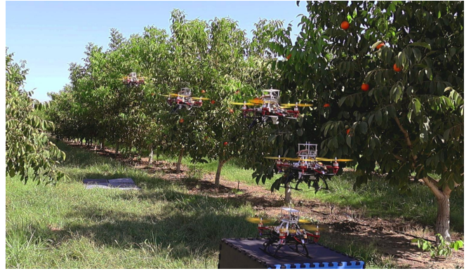
Fig. 1. Experimental vehicle flying autonomously at canopy level while collecting visual data using a RGB camera. This figure is a composite image showing multiple states of the vehicle during flight.
